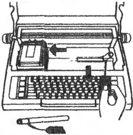
Move carrier to left side of typewriter. Then pull tag hard to remove yellow plastic tube on right side.
